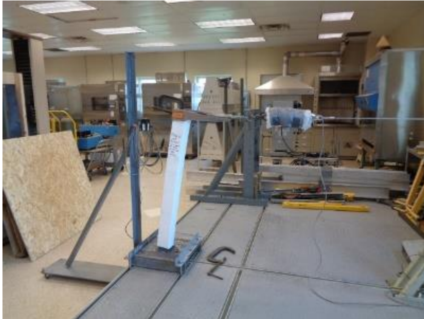
Photo No. 1 Post Mount with Applied Load
