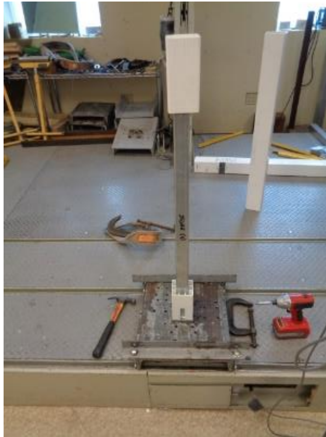
Photo No. 3 Galvanized Post Mount Installed in Simulated Concrete
